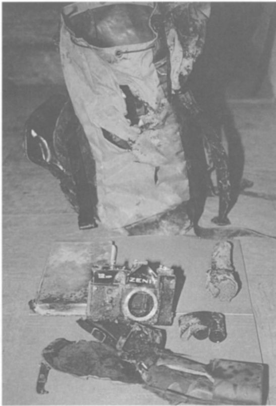
Fig. 6. A backpack, camera with case and film, torch and book were amongst the few items retrieved by search parties. All show thermal damage.
